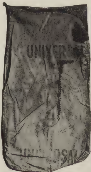
Fig. 4—Extreme care is taken in mending sacks at the Universal Plants. Before making the repair, the cloth is tested to insure sufficient strength, so that often a mended sack is better than one which has passed inspection without needing repair.
